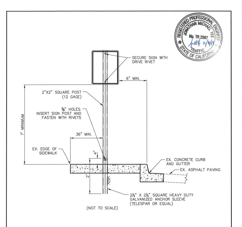
ALL REGULATORY AND WARNING SIGNS SHALL BE MINIMUM 0.063 INCH WITH 3M HIGH INTENSITY PRISMATIC SHEETING (SERIES #3930) WITH 3M PREMIUM PROTECTIVE OVERLAY FILM (SERIES #1160).
